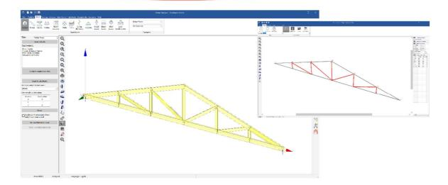
The output for each member includes the graphs showing bending moments and axial force. The calculations and results are printed in the sidebar.
