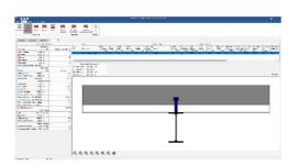
Various spans can be defined, and each span can consist of more than one section. This allows for economical design because you can have a section with reinforcing in the flange to be used in regions of hogging and another without reinforcing in the flange for sagging regions.
